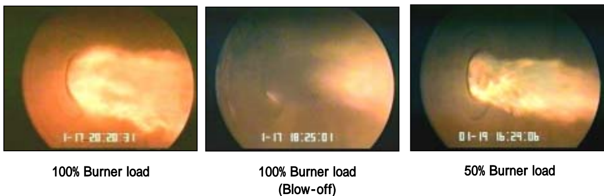
Figure 8. Lignite combustion test flame
